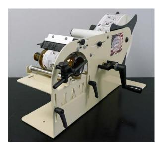
The TAKE-A-LABEL Model TAL-1100M/R Manual Round Product Labeler will label virtually any round product. With just the turn of a handle, labels up to 5" wide can be applied. Products are quickly loaded into the applicator with the unique open carriage design. The top wipe down brush ensures that the labels are fully applied to the product. The open bottle support can be changed from one size to the next in seconds without the use of tools.
