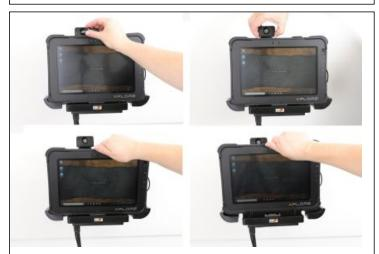
3. Removing the Tablet Turn the key until the center pin pops out on the lock. Slide the lecRolwek upt included to free the top of the tablet.
