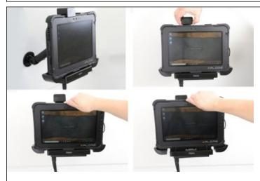
3. **Removing the Tablet** Slide the spring lock up to free the top of the tablet. Pull the top of the tablet forward then lift up to release from the holder.
