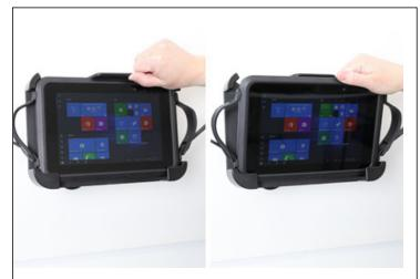
3. **Undocking the Tablet**Using a thumb, press up on the top lip of the holder and then pull forward on the top of the tablet.
